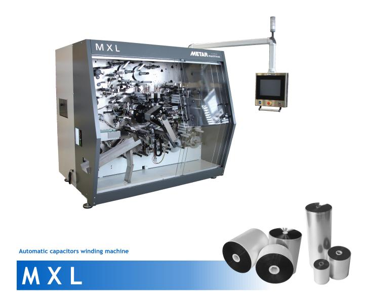
Producing high quality capacitors on plastic core for AC and power electronic applications with concentric winding option
